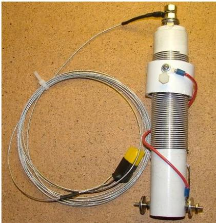
Simply attached the antenna wire to the top of the coil by removing the 5/8 nut slipping the antenna terminal ring over the 5/8 stud and replacing the 5/8 nut. You can hand tighten for portable operation.
