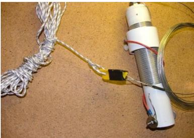
Lastly attach a support to the antenna insulator to a support that can elevate the antenna (like a tree limb). For attic installation you can attach string or other non-conductive support to mount the coil and wire.
