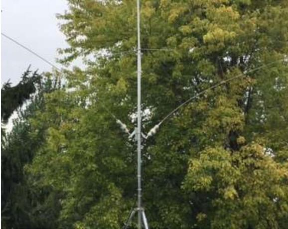
The tuning process stated here is with 102” stainless steel whips. Tuning will vary using longer or shorter whips. Tuning the Otophone is like tuning our Silver Bullet Mini. The difference is you have two coils in a dipole configuration. Put the collars about the same on both coils.
