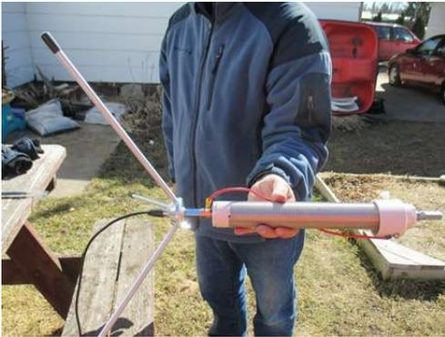
Attach the Silver Bullet 1000 to the coupling bolt.
